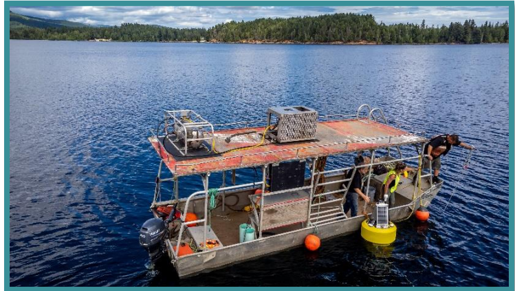
Thermistor buoy deployment on Comox Lake.
