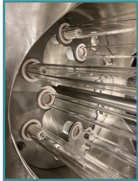
Ultraviolet bulbs inside a reactor.
